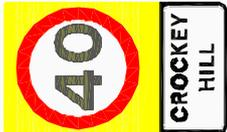
Proposed 'gateway' feature to emphasise the entry into the proposed 40mph speed limit on the A19.
